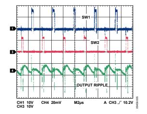
Figure 5. Output Ripple, 50 A Load
