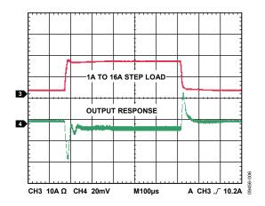
Figure 6. Step Load Transient, Vout
