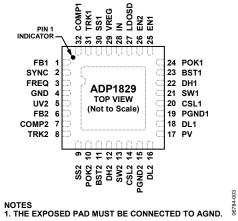
Figure 3. Pin Configuration
