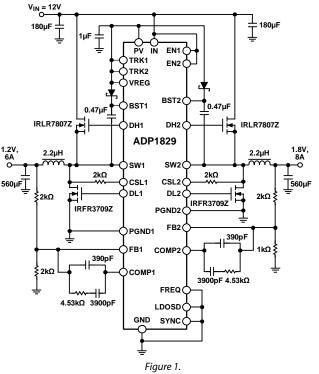
also be synchronized to an external clock to achieve switching frequencies between 300 kHz and 1 MHz. The ADP1829 includes soft start protection to prevent inrush current from the input supply during startup, reverse current protection during soft start for precharged outputs, as well as a unique adjustable lossless current-limit scheme utilizing external MOSFET sensing.
