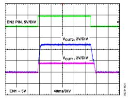
Figure 24. Coincident Voltage Tracking Response
