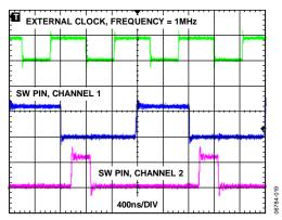
Figure 19. Out-of-Phase Switching, External 1 MHz Clock
