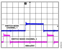
Figure 18. Out-of-Phase Switching, Internal Oscillator
