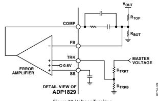
Figure 30. Voltage Tracking
