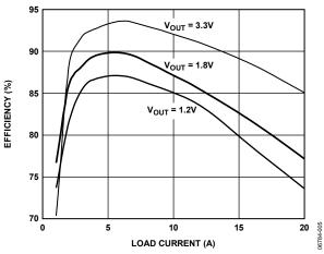
Figure 5. Efficiency vs. Load Current, V<sub>IN</sub> = 12 V, 300 kHz Switching
