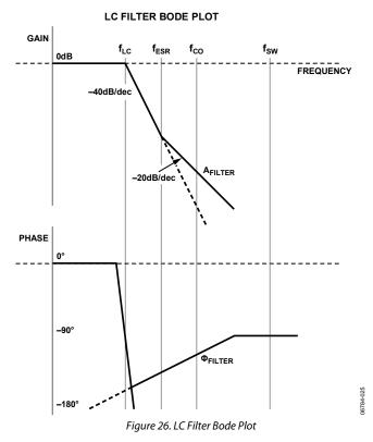
To compensate the control loop, the gain of the system must be brought back up so that it is 0 dB at the desired crossover frequency. Some gain is provided by the PWM modulation itself.
