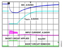
Figure 17. Output Short-Circuit Response
