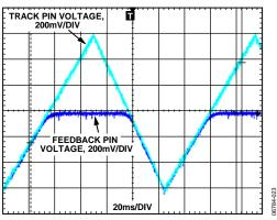
Figure 23. Output Voltage Tracking Response
