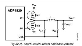
Because the buck converters are usually running fairly high current, PCB layout and component placement may affect the current-limit setting. An iteration of the  $R_{\rm CL}$  or  $R_{\rm LO}$  and  $R_{\rm HI}$  values may be required for a particular board layout and MOSFET selection. If alternate MOSFETs are substituted at some point in production, these resistor values may also need an iteration.
