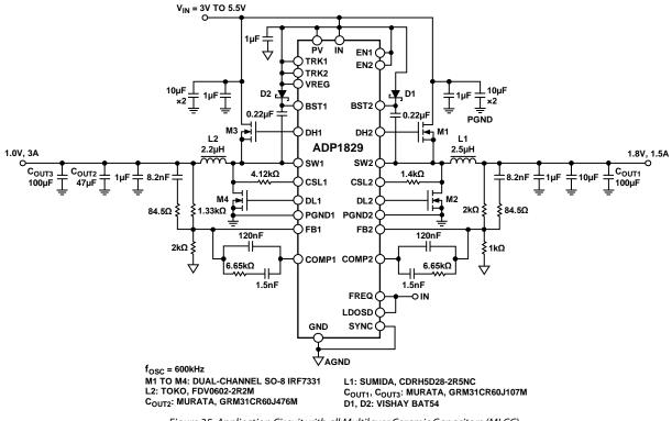
Figure 35. Application Circuit with all Multilayer Ceramic Capacitors (MLCC)
