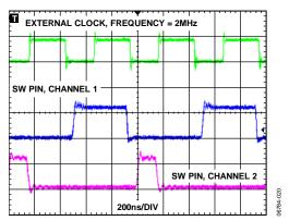
Figure 20. Out-of-Phase Switching, External 2 MHz Clock
