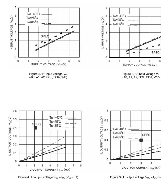
Figure 5. 'L' output voltage VoL – IoL (Vcc=2.5V)
