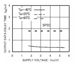
Figure 20. "L" Data output delay time  $t_{PD}0$
