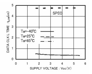
Figure 13. Data clock Low Period  $t_{LOW}$
