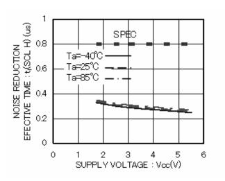
Figure 24. Noise reduction efection time  $t_{\text{I}}\left(\text{SCL H}\right)$
