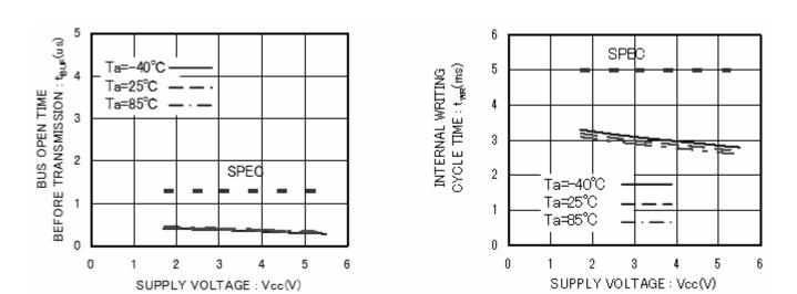
Figure 22. BUS open time before transmission  $t_{\text{BUF}}$
