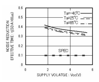
Figure 26. Noise reduction effective time t<sub>I</sub> (SDA H)
