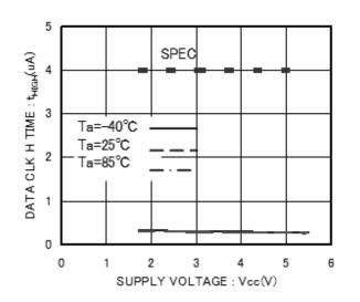
Figure 12. Data clock High Period t<sub>HIGH</sub>
