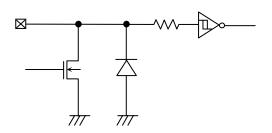
Figure 46. Input /output pin circuit diagram
