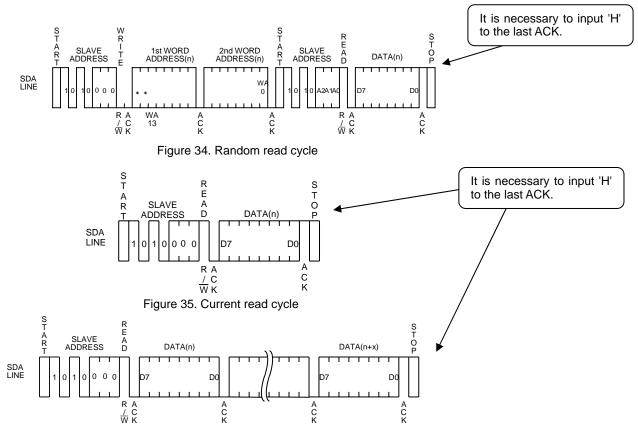
Figure 36. Sequential read cycle (in the case of current read cycle)
