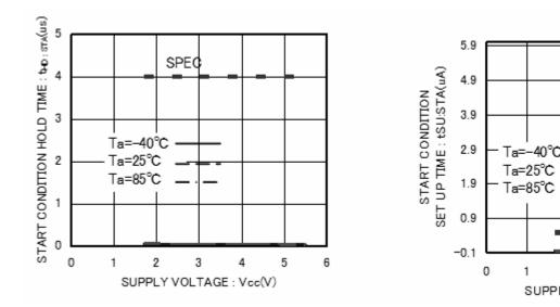
Figure 14. Start Condition Hold Time t<sub>HD:STA</sub>
