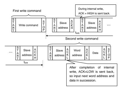
Figure 38. Case to continuously write by acknowledge polling
