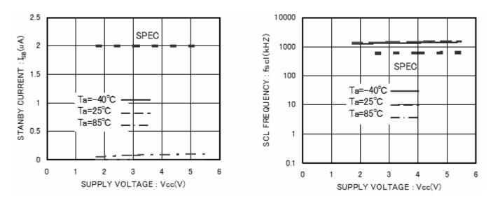
Figure 10. Standby operation I<sub>SB</sub>
