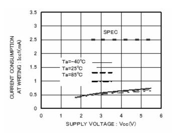
Figure 8. Current consumption at WRITE operation I<sub>CC</sub>1 (fscl = 400kHz)
