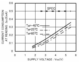
Figure 9. Current consumption at READ operation  $I_{\text{CC}}2$ (fscl = 400kHz)
