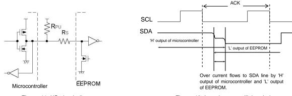
Figure 41. I/O circuit diagram
