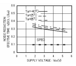
Figure 25. Noise reduction effective time  $t_{l}(\mbox{SCL L})$
