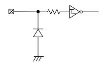
Figure 45. Input pin circuit diagram
