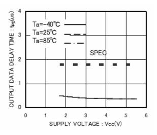
Figure 21. 'H' Data output delay time tPD1
