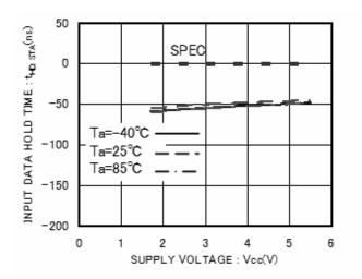
Figure 16. Input Data Hold Time t<sub>HD : DAT</sub> (HIGH)
