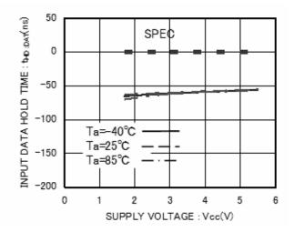
Figure 17. Input Data Hold Time t<sub>HD:DAT</sub> (LOW)
