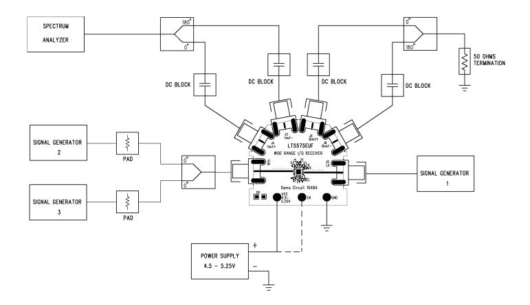
Figure 1. Proper Measurement Equipment Setup
