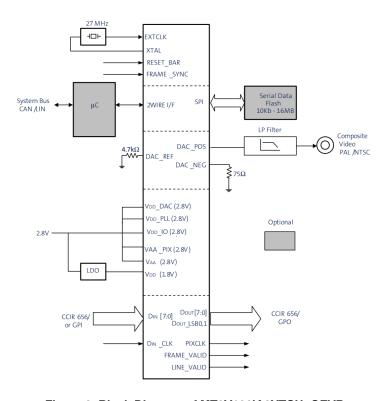
Figure 2. Block Diagram of MT9V126IA3XTCH-GEVB
