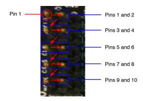
Figure 6. Pin Locations and Assignments of Grouped Jumpers.
