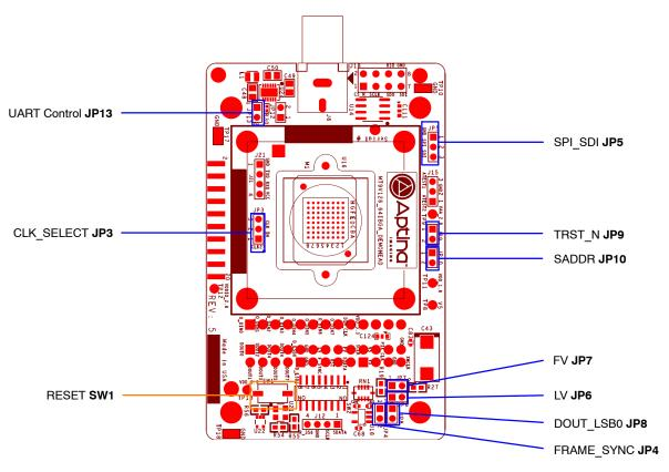
Figure 3. Top View of Evaluation Board – Jumpers
