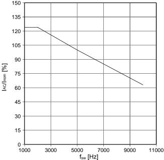
$T_{\text{inlet}}$  - derating curve IGBT (motor), Diode (generator)  $V_{\text{DC}}$  = 750 V,  $V_{\text{AC}}$  = 400  $V_{\text{RMS}}$ ,  $f_{\text{sw}}$  = 5 kHz,  $f_{\text{AC sine}}$  = 50 Hz,  $cos\phi$  = ±0.8 and nom. cooling conditions
