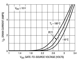
Figure 2. Transfer Characteristics
