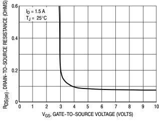
Figure 3. On–Resistance versus Gate–To–Source Voltage
