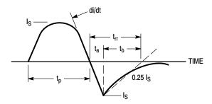
Figure 15. Diode Reverse Recovery Waveform
