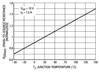
Figure 5. On–Resistance Variation with Temperature
