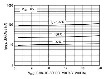
Figure 6. Drain-To-Source Leakage
