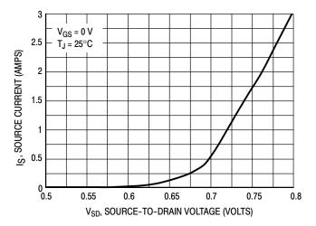
Figure 10. Diode Forward Voltage versus Current
