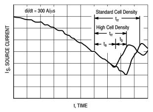
Figure 11. Reverse Recovery Time (t<sub>rr</sub>)
