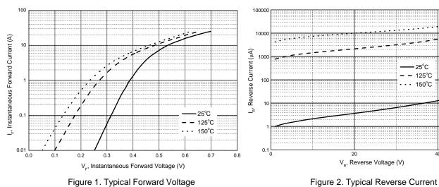
Figure 1. Typical Forward Voltage
