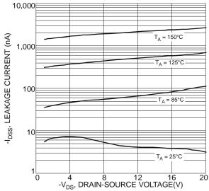
Fig. 13 Typical Drain-Source Leakage Current vs. Voltage
