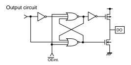
Figure 31. Output circuit (DO)
