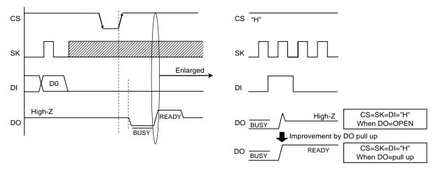
Figure 36. READY output timing at DO=OPEN
