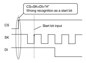
Figure 30. Normal action timing
