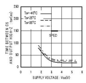
Figure 21. Time from CS to High-Z tDF
