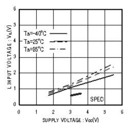
Figure 3. 'L' input voltage VIL(CS,SK,DI)
