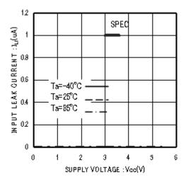
Figure 6. Input leak current ILI(CS,SK.DI)
