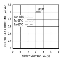
Figure 7. Output leak current ILO(DO)
