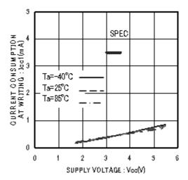
Figure 8. Current consumption at WRITE Action Icc1(fsk=2MHz)
