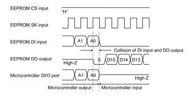
Figure 41. Collision timing at read data output at DI, DO direct connection
