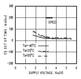
Figure 15. CS Setup time tcss
