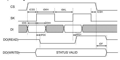
Figure 1. Sync data input / output timing
