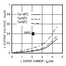
Figure 4. 'L' output voltage VoL-IoL(Vcc=3.0V)
