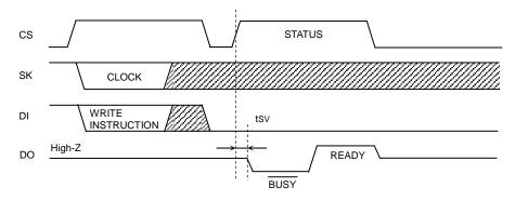
Figure 39.  $R/\overline{B}$  status output timing chart
