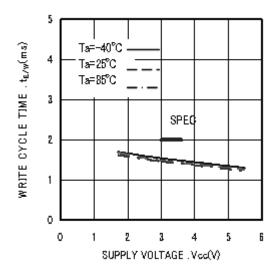
Figure 22. Write cycle time tE/W
