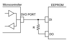
Figure 40. DI, DO control line common connection
