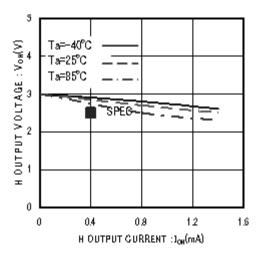
Figure 5. 'H' output voltage Von-Ion(Vcc=3.0V)
