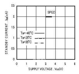
Figure 10. Consumption current at standby action ISB
