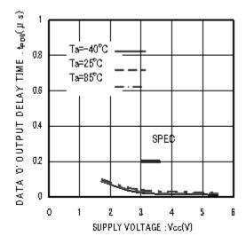
Figure 18. Data '0' output delay time tPD0
