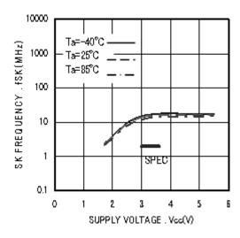
Figure 11. SK frequency fsk
