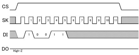
Figure 25. Write enable (WEN) cycle
