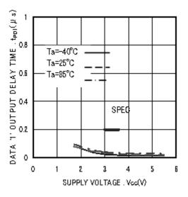
Figure 19. Data '1' output delay time tPD1
